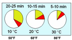
At temperature lower than 10°C (50°F) the hardening can be not homogeneous and even with consequent decrease of the mechanical properties of the hardened adhesive
